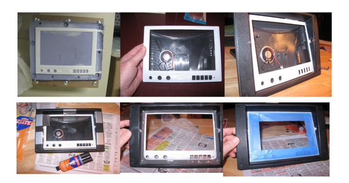
I used a combination of Loctite Epoxy Gel (to initially adhere the two bezels together), epoxy putty (to fill the majority of voids), and JB Weld (to have a nice fluid finish along the top surface). There are a few pictures below. I didn't do a final fill of some of the voids because I know that the process will work, so I painted it to get a general idea of the finished bezel.
